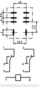
MOUNTING HOLES & BOTTOM VIEM LY3,-S,-N,-F,-O ЎЎЎЎĽY4,-S,-N,-F,-O
